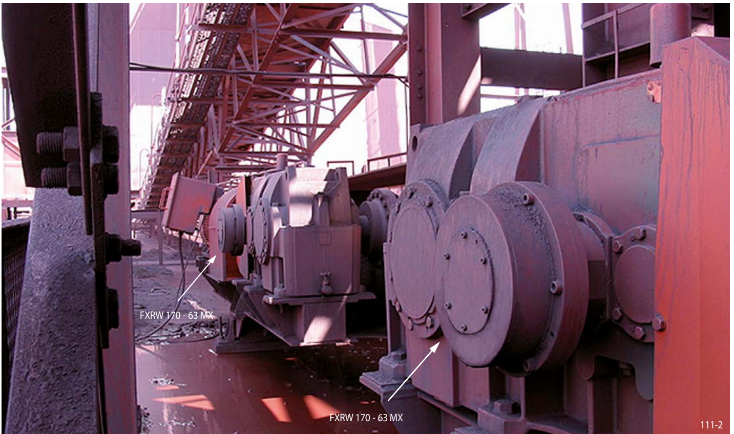
Iron ore conveyor plant in South Africa driven by three gear reducers with RINGSPANN backstops FXRW 170-63 MX.
